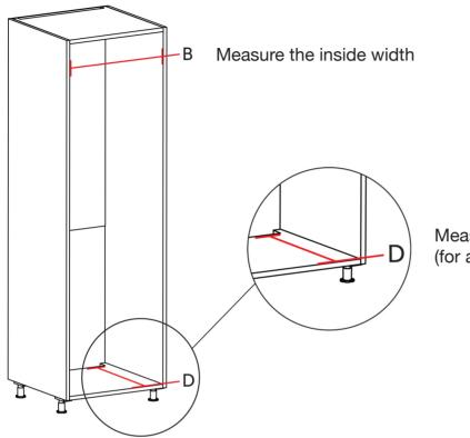
Measure from the back opening (for airflow) to the front ledge
