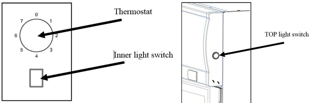
The first time you put your appliance into operation, set the thermostat to the middle position "4" and let it run empty for 4 hours for it to cool down sufficiently.
