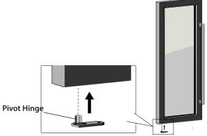
**12**.Install the door to the left hinge side by tightening the Pivot Hinge with the 2 screws.
