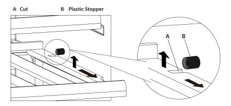
• For a model with Telescopic Rail, pls. lift the whole Shelf upwards horizontally to get it off from the 4 Locating Pins of Telescopic Rail.
