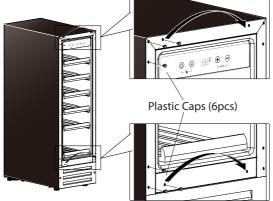
**5.**Install the Upper Left Hinge and Bottom Left Hinge to the left side of the cabinet. Make sure the screws are tightened.
