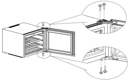
o Unscrew the 3 screws from Top Bracket, move the bracket to the right end and screw the 3 crews.
