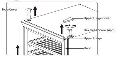
**2.**Move the Hinge Hole Cap (at the top of the door) from the left side to the right side. Move the Pivot Hinge (at the bottom of the door) from the right to the left side.
