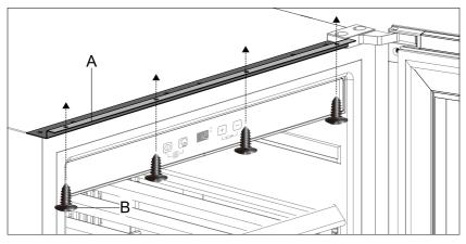
A. Top Bracket B. <sup>4</sup> Screws (ST<sup>4,2\*12</sup>mm)
