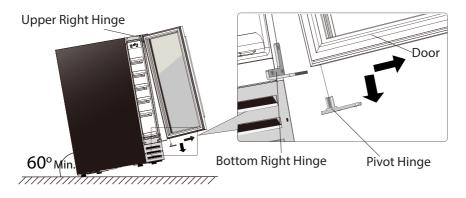
**3**. Unscrew the Upper Right Hinge and Bottom Right Hinge from the cabinet. Keep them well for door re-installation.
