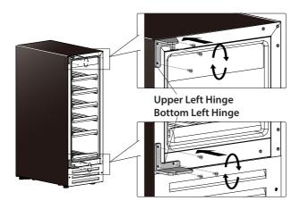
**6.**Move the Hinge Hole Cap (at the top of the door) from the left side to the right side.
