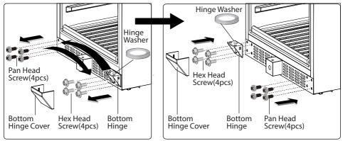
**4.**Hold the Door carefully with your assistant and place it on the top of Bottom Hinge , make sure the Pivot Hinge is at correct place through the Hinge Washer. Insert the pin of the Upper Hinge into the Bushing on the top right and fix it with Hex Head Screw (4pcs). Cover the Upper Hinge and Bottom Hinge with Upper Hinge Cover and Bottom Hinge Cover. Cover hinge screw holes on the top right with the Hole Cover.
