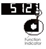
o When the compressor starts to work, the Indicator will stay on;
