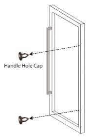
**8.**Gently pull the door gasket to one side to reveal the Handle Screws (2pcs) on the left side of the Door.Unscrew it with a cross screwdriver and Remove the Handle (Leave the Washers as where it is).
