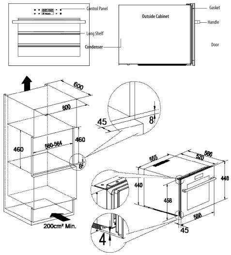
For a firmly fixing of the unit you can install an extra **Top Mounting Bar** (which is an accessory packed with the unit) onto the topside of the unit and screw it with the kitchen cabinet. See right drawing.
